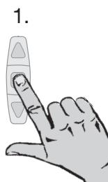
When the required intermediate position has been reached, keep the **STOP** button depressed and, if necessary, correct the position with the **UP** or **DOWN** button. Release the **STOP** button when the exact position has been reached.
