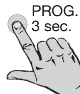
Within approx. 4 minutes, press the **PROG** button for the new transmitter for 3 seconds (wait until the transmitter control light flashes **once**).
