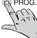
Then press the **PROG** button of the transmitter to be deleted for a short time. The relevant transmitter has now been deleted from the receiver.
