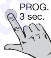
When one transmitter has already been learnt, press the **PROG** button for 3 seconds (wait until the transmitter control light flashes **once**). Then the receiver will be in programming mode for 1 minute.
